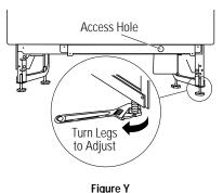
TIP: Pull lower rack out, about halfway. Check to be sure the rack does not roll forward or back into dishwasher. If the rack rolls in either direction, the dishwasher must be leveled again.
